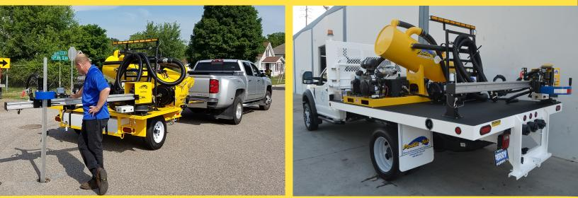
These units are offered as a skid mounted vacuum or can be built onto a flatbed or trailer. Pacific Tek offers seven basic tank sizes with over 100 different configurations and options, depending on the customer's needs. The larger tanks have a reverse flow option where, at the flip of a lever, flow is reversed in the system which allows you to either pump liquid or slurry out of the tank to a higher place, or, to free up clogging in the pickup hose by having air blow the reverse direction.
