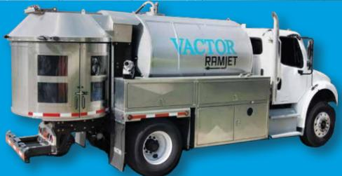
Instituting a regular line maintenance program is easy with the Ramjet 850 truck-mounted jetter. Equipped with the Vactor JetRodder water pump, the Ramjet effectively breaks up blockages in sanitary lines, flushes out debris and scours sewer lines clean.
